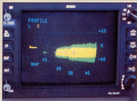
Leather seats and plenty of room distinguish the Mirage's cabin. An AlliedSignal RDR-2000 with vertical profiling is also standard.
